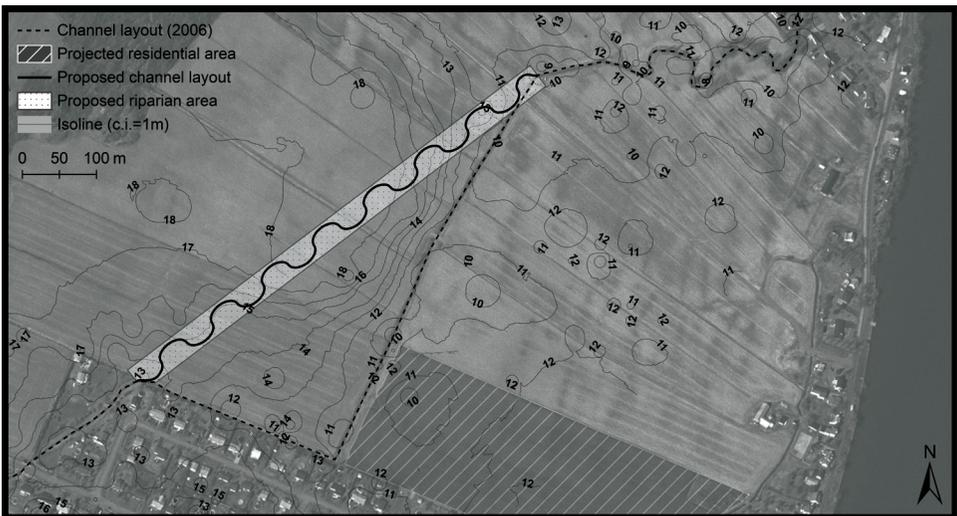
Figure 8. Potential solution relying on the migration of part of the Richer channel from the residential area to an agricultural zone to limit bank erosion and flooding problems in the residential sector.
