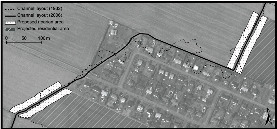
Figure 7. Potential solution consisting in the naturalization of two parts of the Richer channel that are located near future residential developments. The width of the riparian zone for the two proposed development is based on the natural (1932) meander amplitude for each zone.
