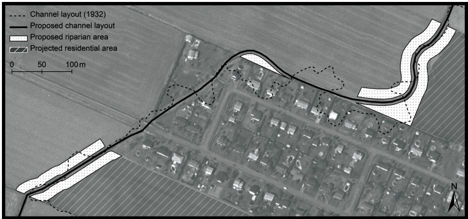
Figure 9. Potential solution relying on planform and shape alterations, stabilization with vegetation and bioengineering techniques, and naturalization.
