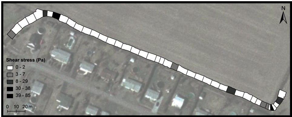
Figure 4. Estimated bed shear stress values in the residential reach. Flow is from left to right.
