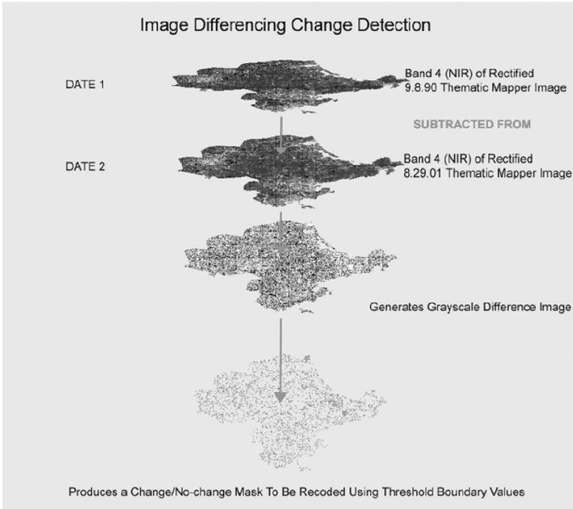
Figure 3. Procedural steps in performance of the Image Differencing Change Detection technique.
