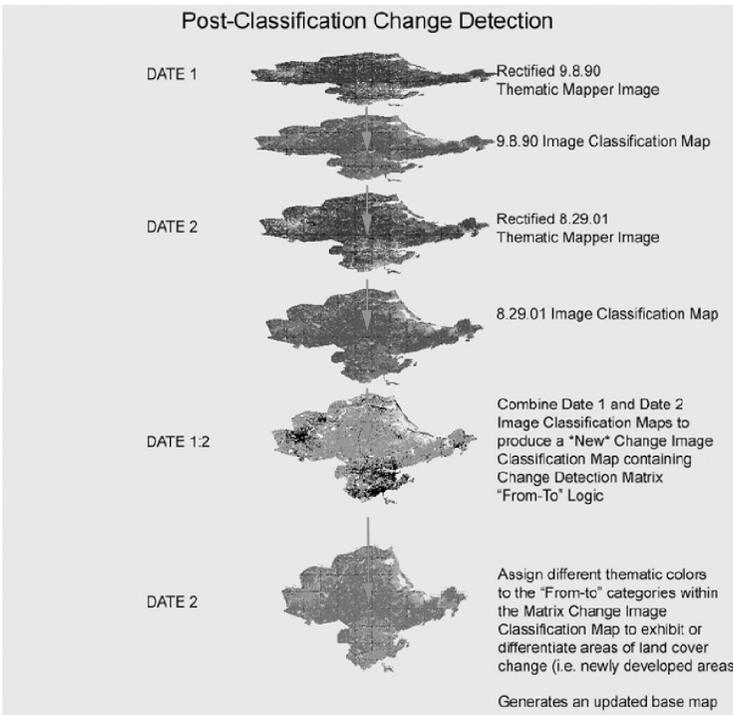
Figure 4. Procedural steps in performance of the Post-Classification Change Detection technique.
