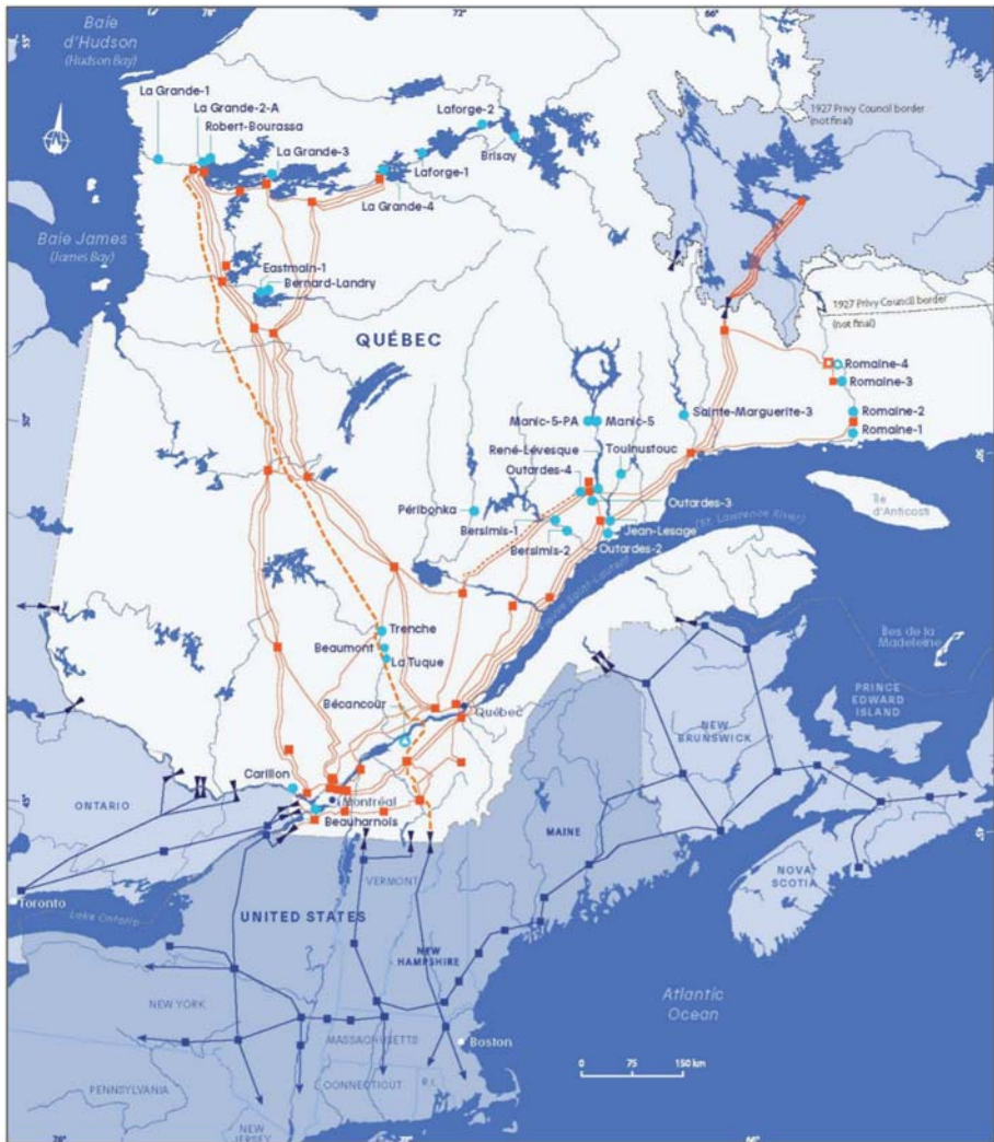
Figure 3. Hydro-Québec's transmission grid, showing high-voltage interconnections to neighboring provinces and states (Hydro-Québec 2021).
